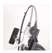
The top chain rings utilizes a manual shifter system located on upper crank which minimises cables and maintenance.
