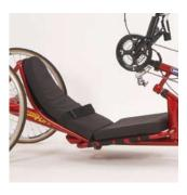
Adjustable back angle allows you to recline the back from 35-55 degrees.
