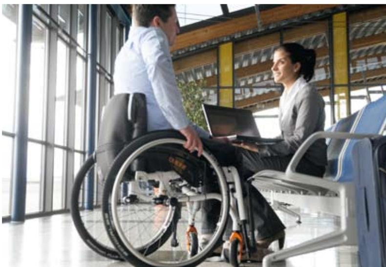
\* 40 x 40 cm; low frame; slim style sideguards; 24" Proton wheels + aluminium handrims; 3" castors; angle adjustable back; 35 cm fixed height backrest; compact wheel lock; no pushhandles + lightweight backrest upholstery; flip-up footrest
